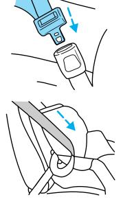
6. Allow the belt to retract to remove slack. The belt will click as it retracts to indicate it is in the automatic locking mode.
